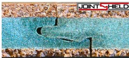
Penetration of the protective sealant into the core board of the GFIX profile.
