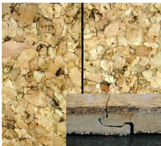
difference between a GFIX edge protected with JOINTSHIELD and a standard competition joint when both were under water for 24 hours.
